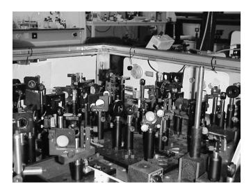
The pulse-generation part of the experimental setup (schematic picture in Fig. 2.2 on page 21). The two white boxes at the right are two TOPASES. As an indication of the scale for those who are not familiar to optical experiments: most objects are about 15 cm in height.
